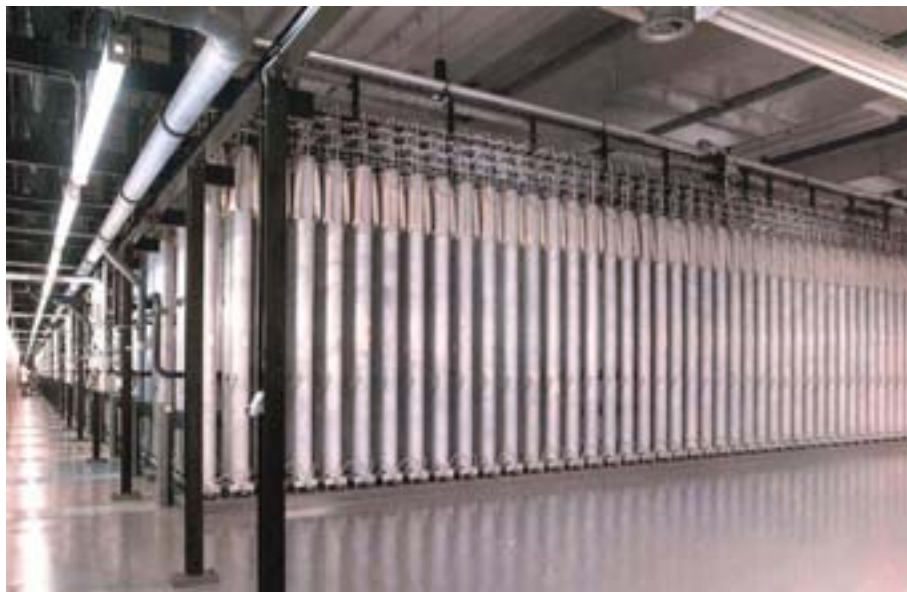
Centrifuge enrichment, at Urenco in Gronau, Germany (photo courtesy of Urenco Germany).
