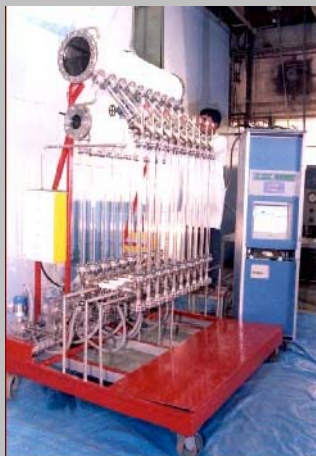
Transparent Setup for Natural Circulation Flow Distribution Studies
