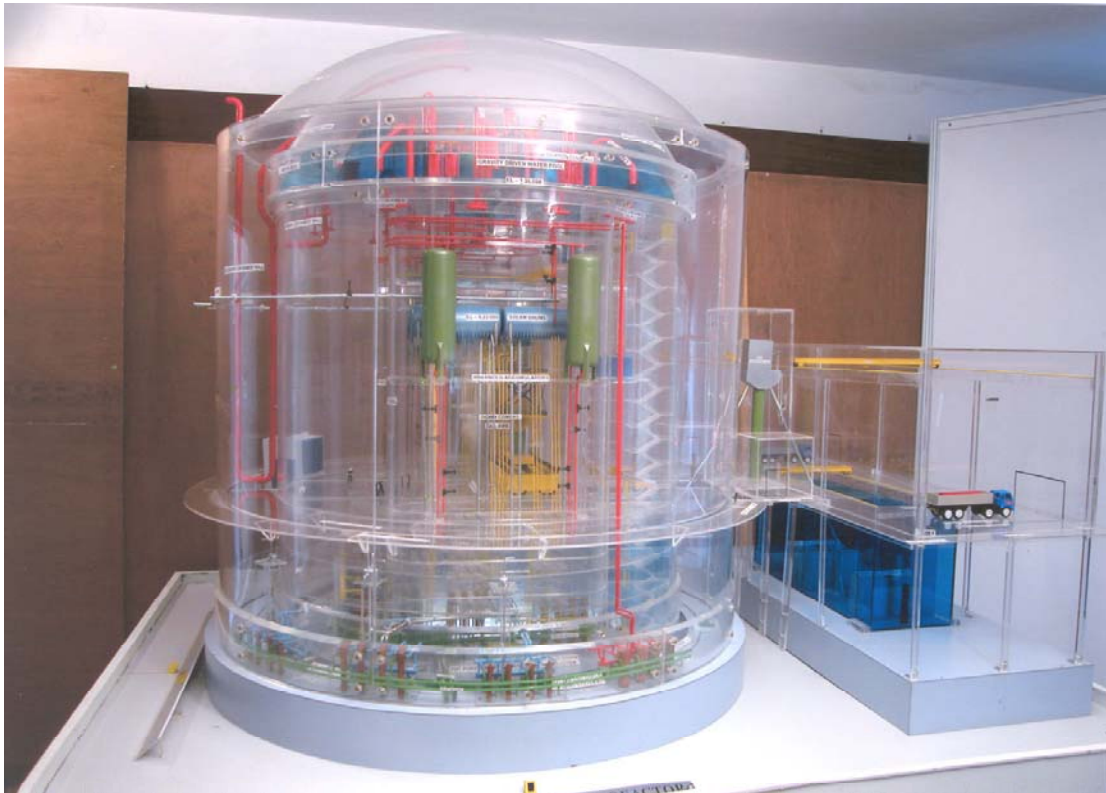
An Acrylic Model of AHWR to Scale 1:50
