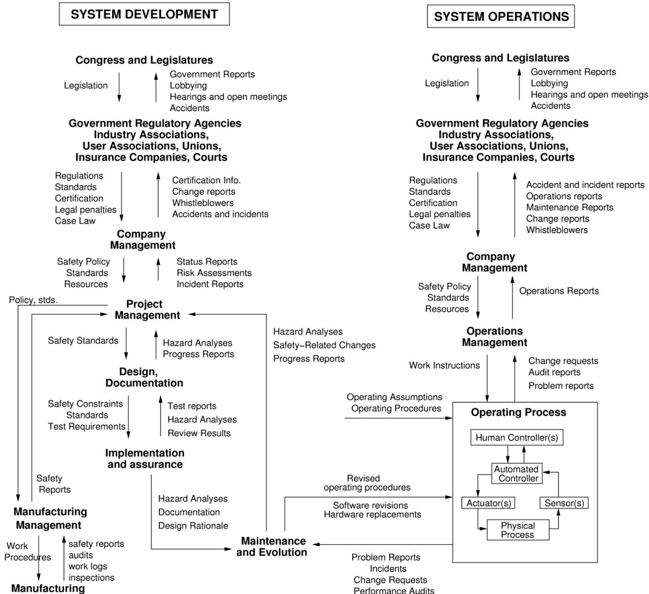
Figure 1. Generalized control structure diagram [from Safer World, Nancy Leveson].
