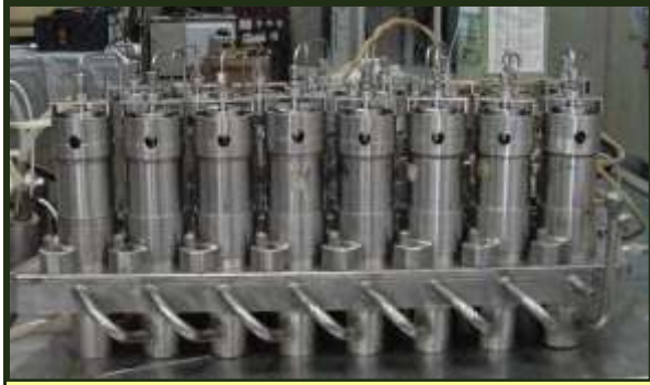
16 Stage Centrifugal Extractor Bank
