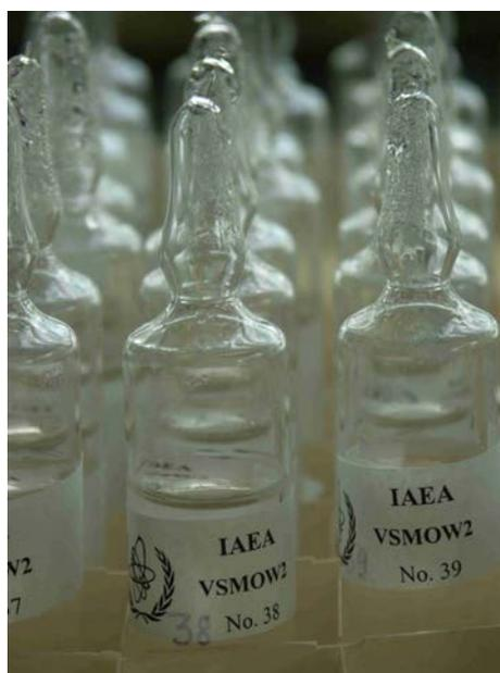
Fig.2: Sealed 20mL glass ampoules as used by IAEA for long term storage of water reference materials.
