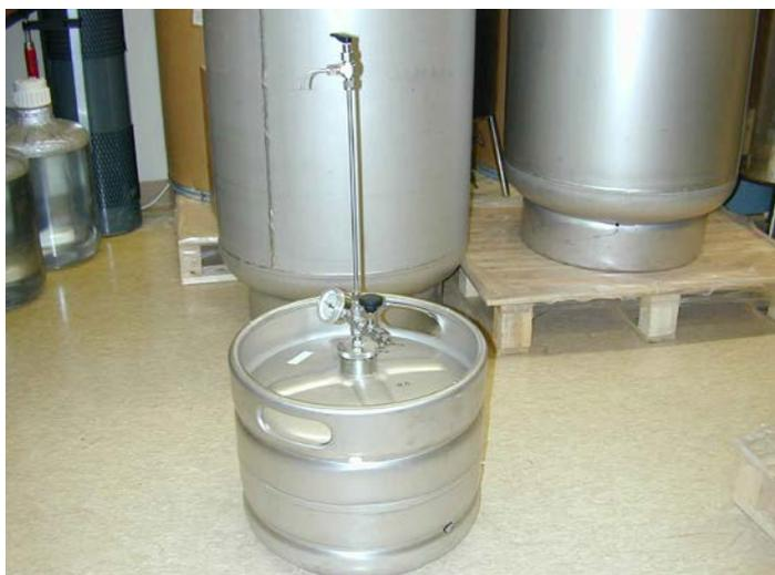
Fig.3: Stainless steel tank for storage of water internal laboratory standards with water dispensing assembly.
