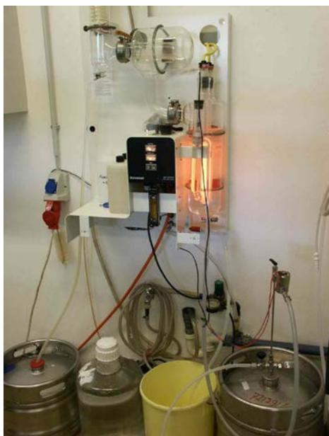
Fig.1: Modified commercial distillation unit for distillation from a closed tank (lower right side) into another tank at lower left side, to minimise any isotopic change of the water during distillation.
