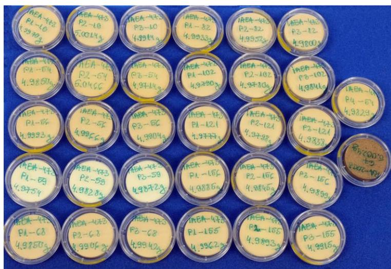
*FIG. 4. Pellets from milk powder produced by high pressure equipment*
