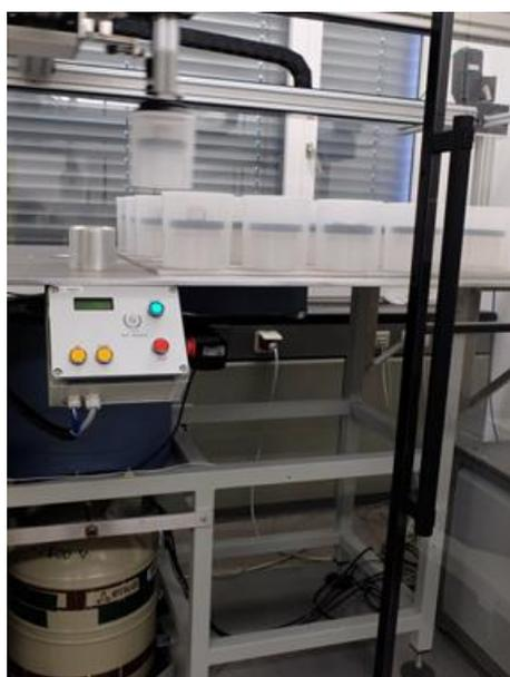
FIG.5. Automatic sample changer
