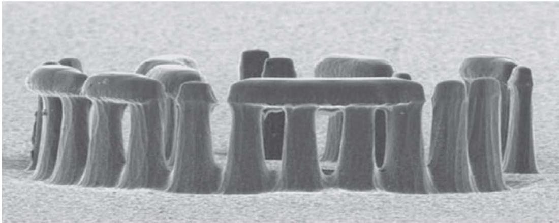
**Figure 4: Stonehenge micromachined in silicon: 80  $\mu\text{m}$  diameter**
