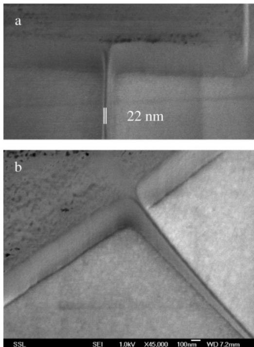
**Figure 3: 22 nm line in 850 nm HSQ by Proton Beam Writing**
