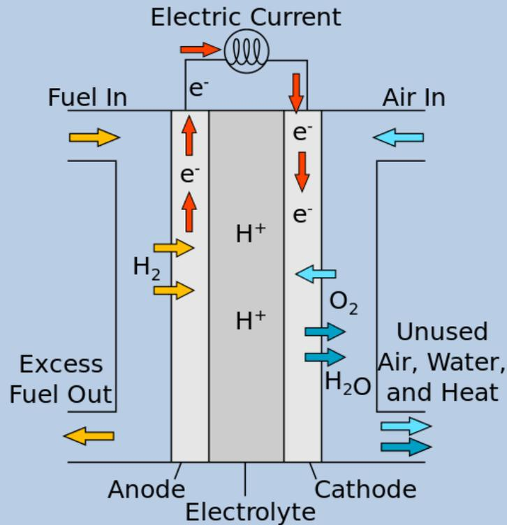
The system can be easily scaled by having flow plates with multiple hydrogen channels on the anode side, and multiple air channels on the cathode side.
