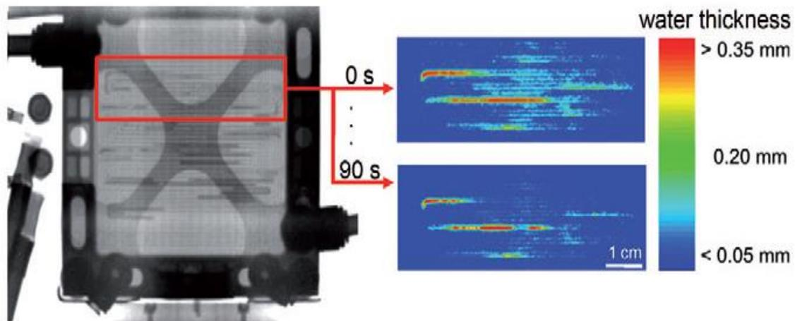
**Water distribution in a fuel cell. At 0 s the fuel was changed from hydrogen to deuterium.**
