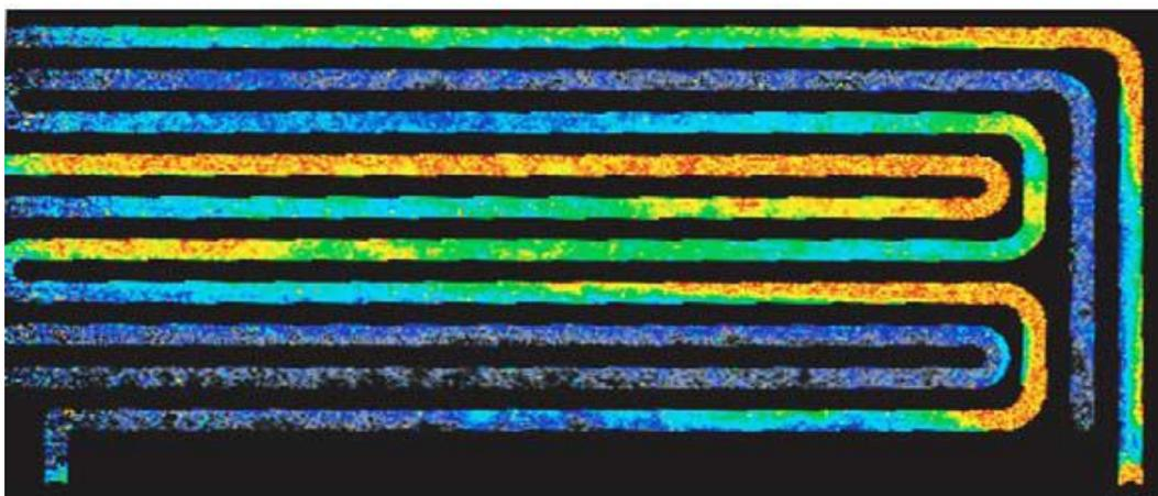
**Water in the cathode side of a fuel cell.**
