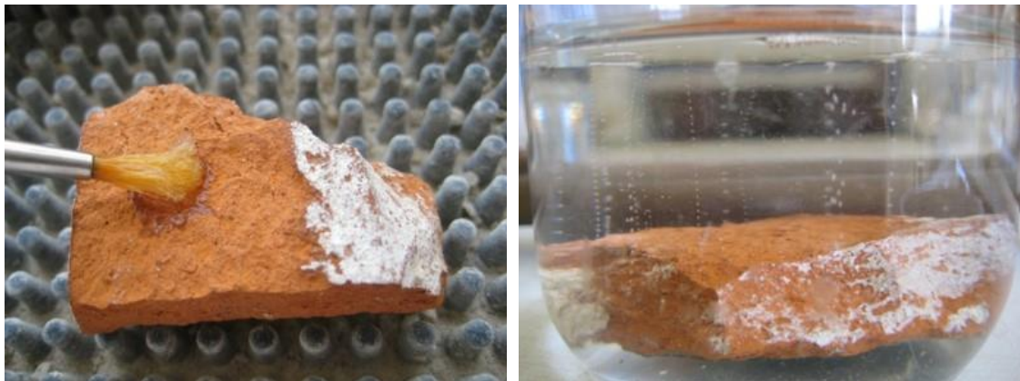
Photographs of the brushing (left) and immersion (right) techniques for the application of resin in the a green glazed tile from the “Madre de Deus” Church, “Museu Nacional do Azulejo (MNA)” (Lisbon, Portugal). Figure credit: Adapted from M.I. Prudêncio et al., 2012.
