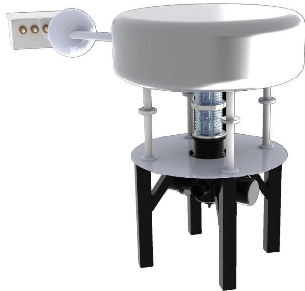
240 kV ESQ Accelerator
