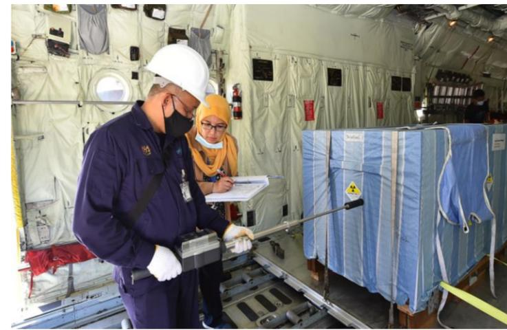
*Monitoring radiation exposure inside the plane.*
