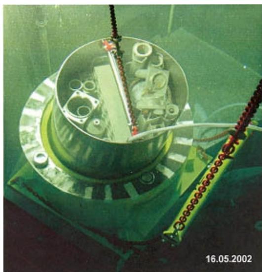
Figure 4. Conditioning of ILW – Under water loading of GNS-Mosaik Container
