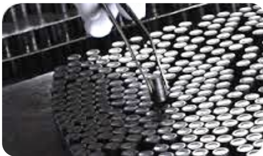
Fig. 1: Due to the negligible sampling uncertainty associated with the stable and homogeneous material in sintered pellets, pellet samples are regularly taken for DA to monitor the quality of the operators' measurement system at fuel fabrication plants.
