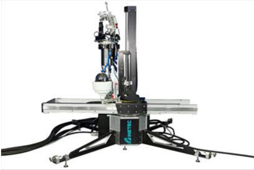
FIG. 46. Example of a RPVH inspection probe manipulator.
