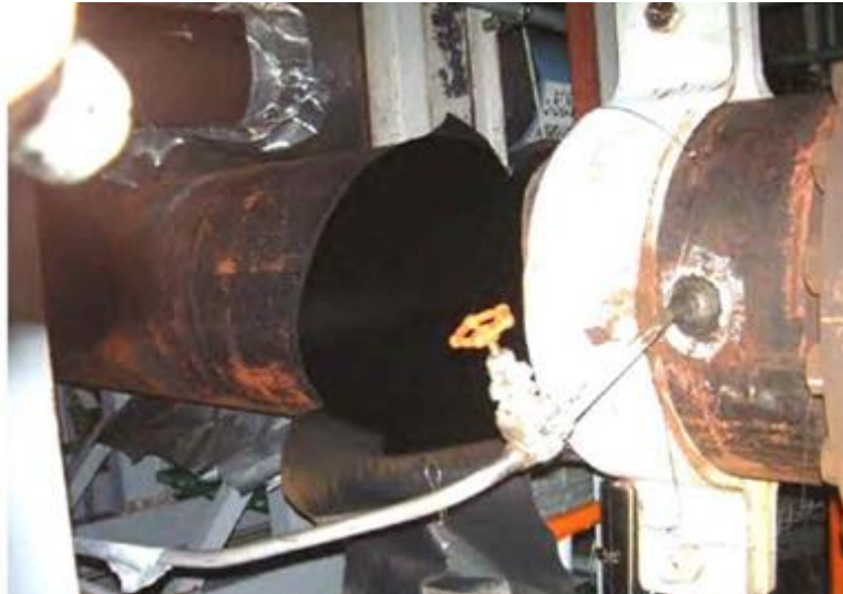
FIG. 37. A 56 cm catastrophic rupture in the condensate line downstream of an orifice in the Mihama nuclear power plant in Japan [61].
