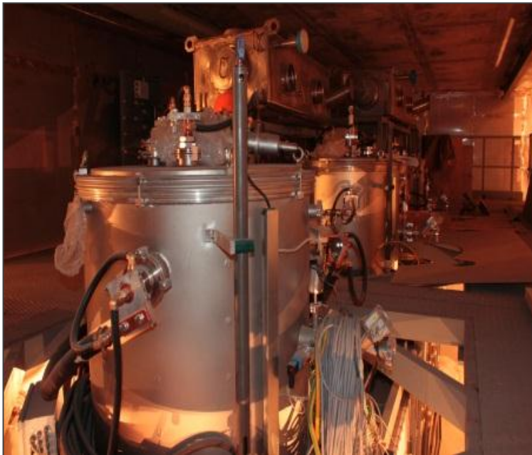
System for fuel pellets sintering, MOX fuel fabrication
