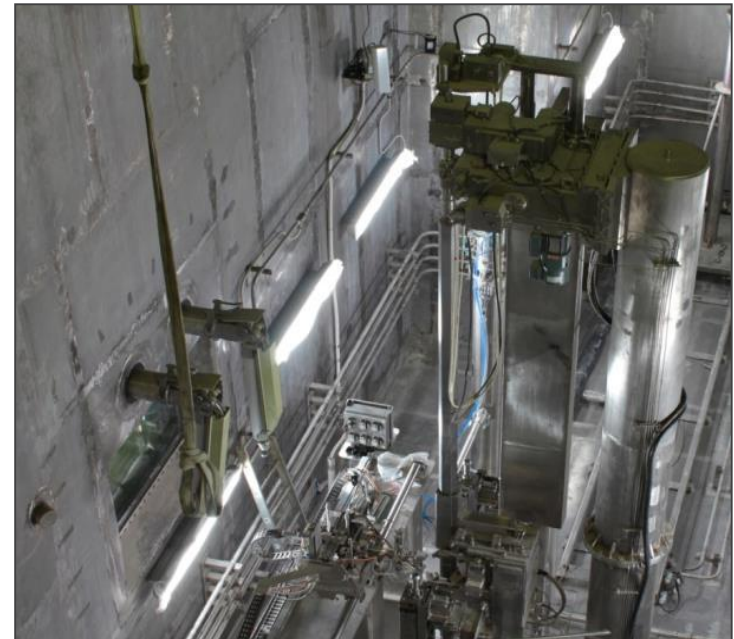
System for assembling fuel rods into the final fuel assembly structure
