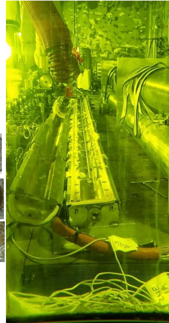
7-zone full length fuel rod heater
