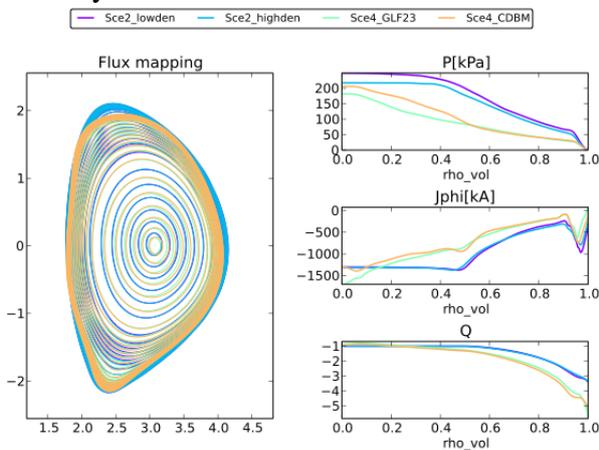
FIG. 8 JT-60SA magnetic equilibria produced by CHEASE, pressure, toroidal current and safety factor ( $Q$ ) profiles for the four scenarios (all obtained with GLF23[34] transport model, whereas Scenario 4 was also run with CDBM[35]).
