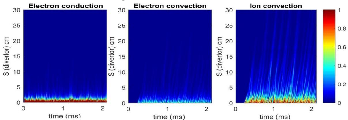
FIG 10 Electron conductive, electron convective and ion convective power depositions (in  $\text{MW/m}^2$ ) on the divertor surface from an HESEL simulation using experimental ASDEX Upgrade parameters for a connected divertor case. The figures show the radial variations in a time span of 2.1msec ( $S$  is the coordinate along the divertor surface).
