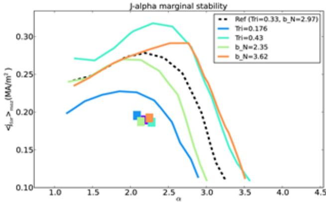
FIG. 7 Marginal stability curves (obtained at  $\gamma\tau_A \sim 0.02$  to account for diamagnetic stabilization contribution) for EU DEMO1 2015 scenarios (reference scenario in dashed line; operational points in squares), varying triangularity or core plasma beta (at constant pedestal profile and total current).
