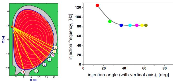
FIG. 5 Left: pellet injection angles, varied between  $10^\circ$ - $70^\circ$  (versus vertical axis), for a same entry point at the vessel. Right: pellet injection frequency adjusted by the controller as a function of injection angle. For trajectories 1-2 the deposition shifts outwards, fueling is less efficient, forcing the controller to increase the injection frequency in order to maintain the required density.
