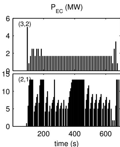
FIG. 3: EC feedback power needed to stabilize NTMs and maintain their size below the critical size, in the case of 5s time step.
