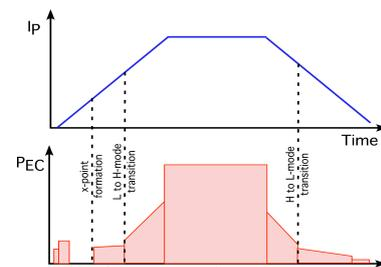
*FIG. 1: Schematics of the applications of the Electron Cyclotron system during the various phases of a plasma discharge [1].*
