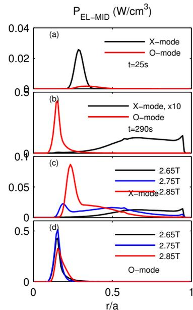
FIG. 4: Power density profiles from the EL-MID launcher ( $R = 9.394\text{m}$ ,  $z = 0.62\text{m}$ ), at 2.65T (a) in L-mode, (b) in the flattop (power in X-mode multiplied by a factor 10), and for different values of magnetic field for (c) X-mode and for (d) O-mode polarization.
