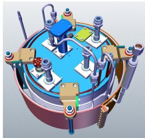
Fig. 3. EM shield with RF driver.
