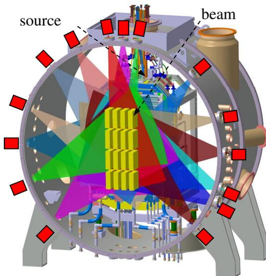
*Fig. 3. Vertical cross-section of the SPIDER vessel with view of the 4x4 beamlet groups and 15 linear cameras of the tomographic diagnostic with corresponding fans of lines of sight*
