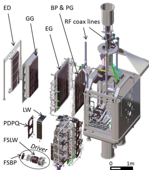
Fig. 1. Beam Source 3D exploded view.
