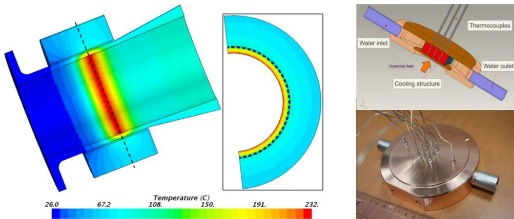
*FIG. 1. On the left side, the predicted temperature field on the solid structure of a gyrotron cavity cooled with mini-channels; on the right side, schematic view and photograph of a thermal cavity mock-up to be tested in the AREVA electron beam test facility.*
