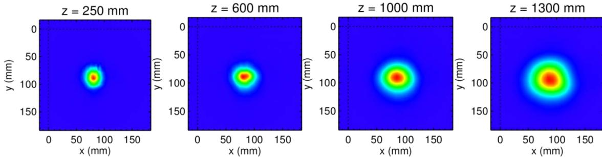
Fig. 5. IR images of the RF output beam profile measured on a PVC target at 250 mm, 600 mm, 1000 mm and 1300 mm from the window respectively.
