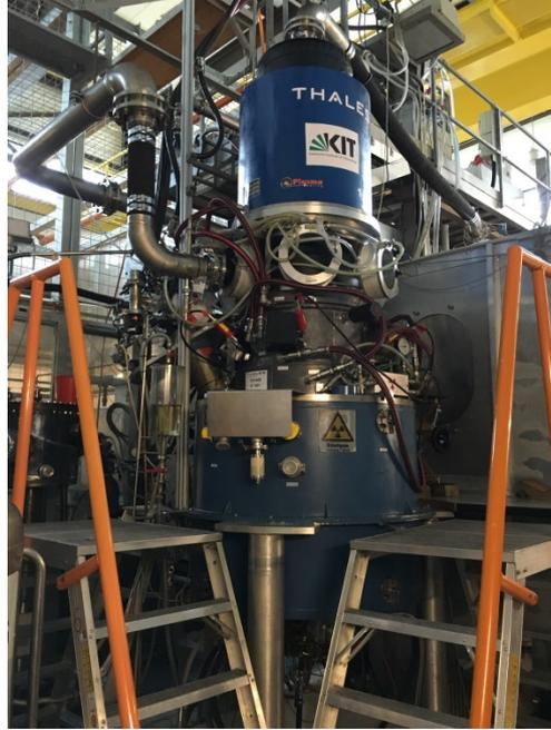
FIG. 3. The 1MW CW gyrotron assembly at the KIT test facility.
