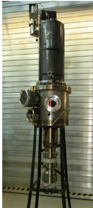
*FIG. 1. The short-pulse gyrotron installation at KIT for RF testing.*
