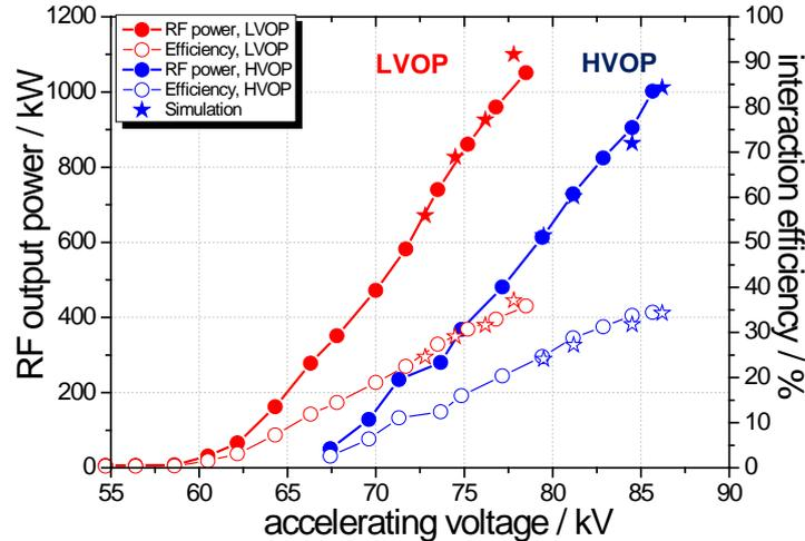
FIG. 2. Output power in the  $TE_{32,9}$  mode vs accelerating voltage, as simulated (stars) and experimentally measured (circles) for the LVOP and HVOP operating points of the SP gyrotron.
