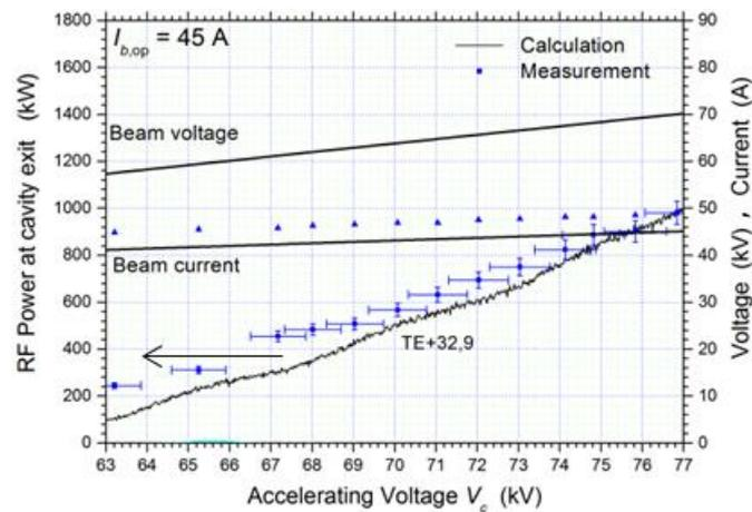
FIG. 4. Comparison between experimental results (in blue) and simulation results from the multi-mode code EURIDICE (in black) at the LVOP for an electron beam radius of 9.55mm and a magnetic field angle at the emitter of -2 deg.
