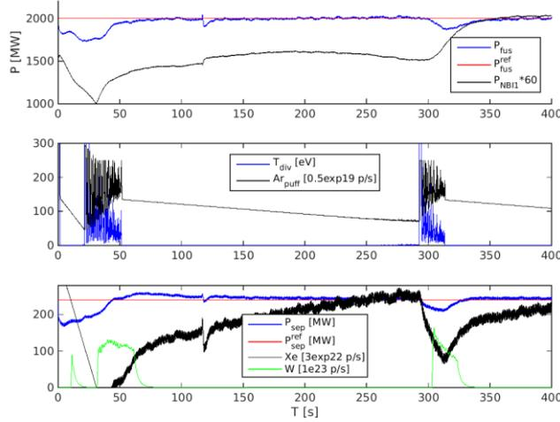
FIG 4. Example of simultaneous fusion power and divertor detachment control. In the central plot, the Ar puff increases when the divertor detachment is lost. Loss of detachment causes an increase of W erosion at the plate (bottom), which requires the intervention of NB to maintain the fusion power at the required level of 2 GW (top) to contrast dilution. The coupling ASTRA/divertor model is described in [33,34].
