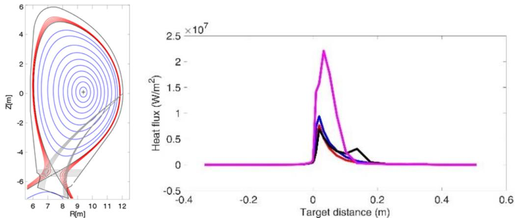
FIG 3.(left) Example of lines of sight for the divertor detachment diagnostic.)
