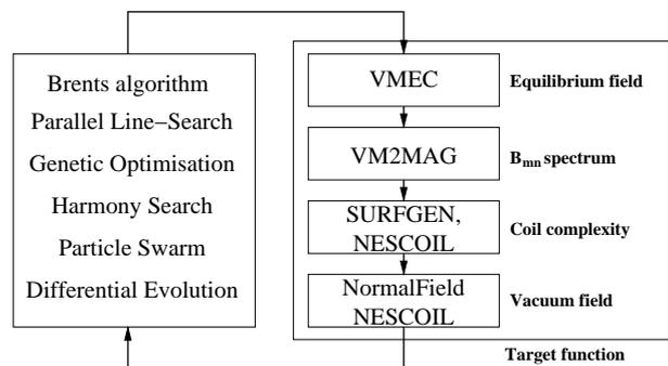
Figure 1: Procedural structure of the ROSE code.
