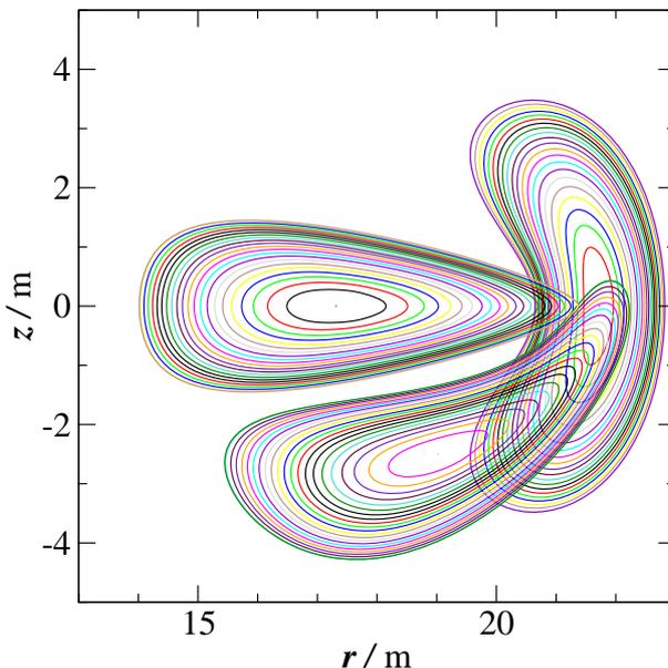
Figure 4: Cuts of the the flux surfaces of a quasi-helically symmetric configuration at selected toroidal angles.
