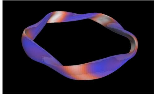
Figure 2: Optimised plasma boundary of a QI configuration at  $A = 12.2$ . The magnetic field strength is color coded.
