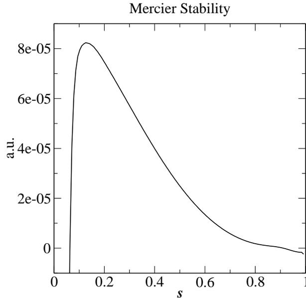
Figure 5: Mercier plot from VMEC data for a qh-symmetric configuration. Positive values indicate stability.
