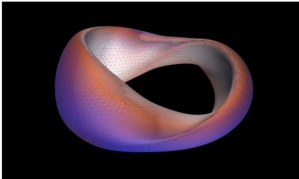
Figure 3: Plasma boundary of a quasi-axially symmetric stellarator with the magnetic field strength colour coded.
