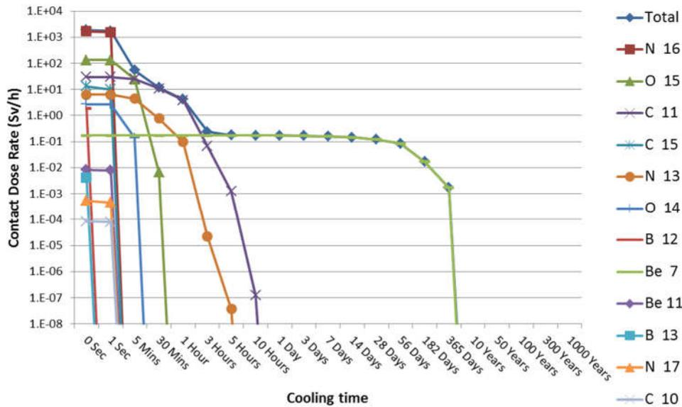
FIG 8. Time evolution of the principal radionuclides in terms of contact dose rate calculated for the TC cooling water in the most inner layer
