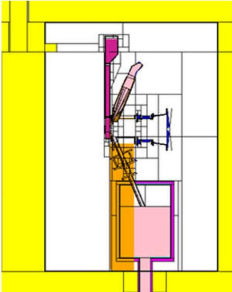
FIG. 1. Test Cell MCNP model used for calculations. Biological shielding are is colored in yellow.
