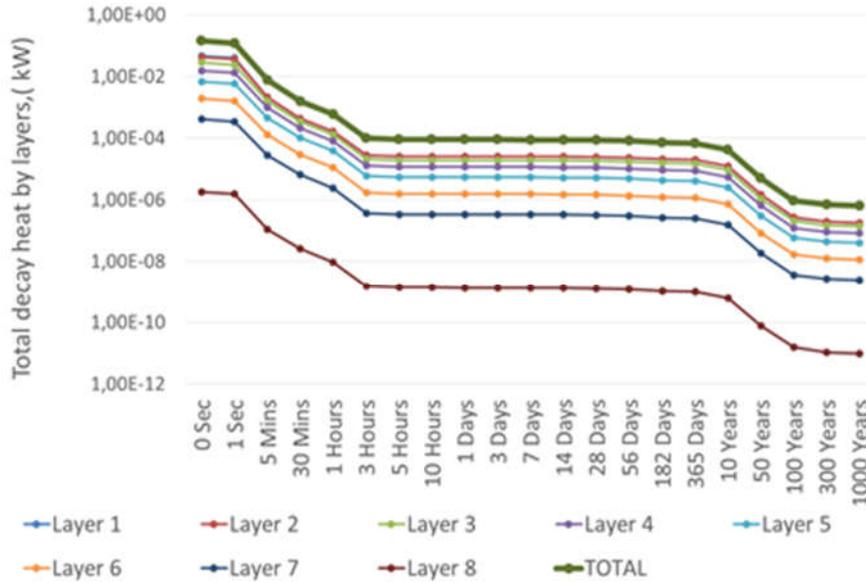
FIG. 5. Total decay heat of cooling pipes present in different layers
