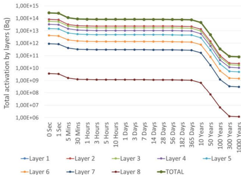
FIG. 4. Total activity of cooling pipes present in different layers
