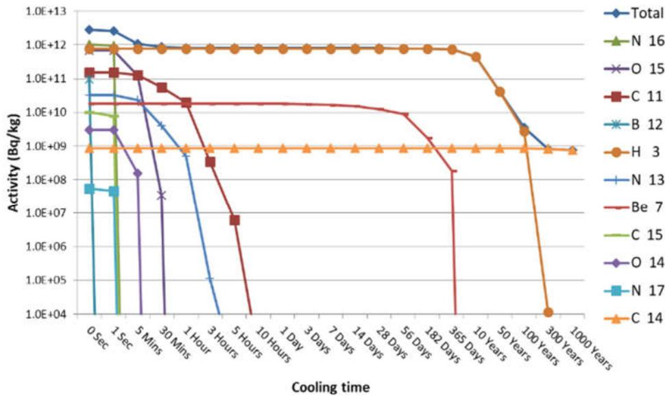
FIG 6. Time evolution of the principal radionuclides in terms of activity calculated for the TC cooling water in the most inner layer
