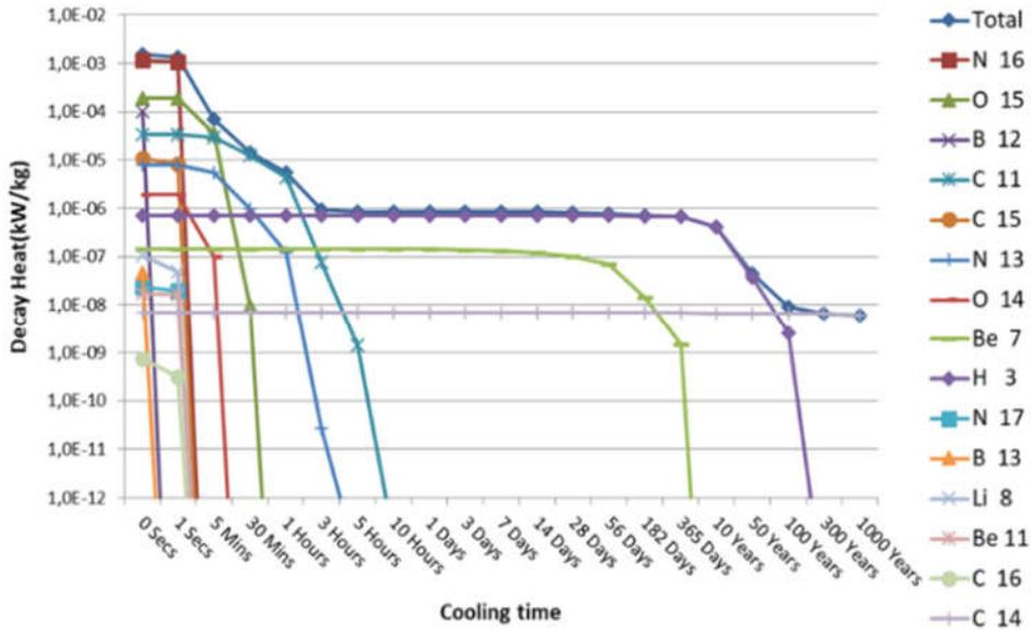
FIG 7. Time evolution of the principal radionuclides in terms of decay heat calculated for the TC cooling water in the most inner layer
