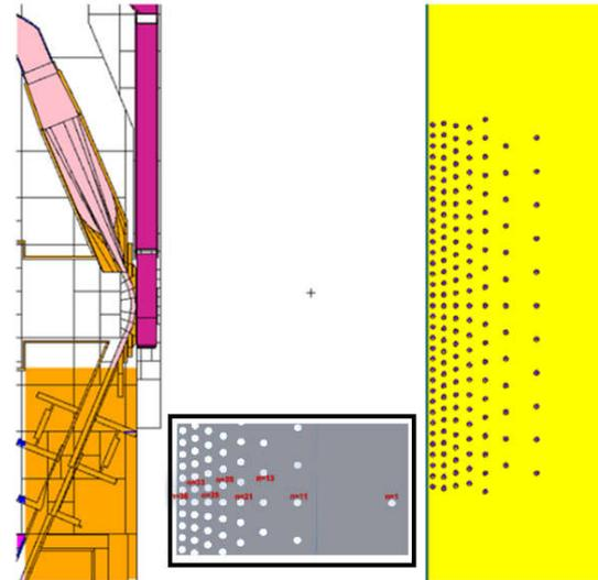
FIG. 2. Pipe placement inside the biological shielding.
