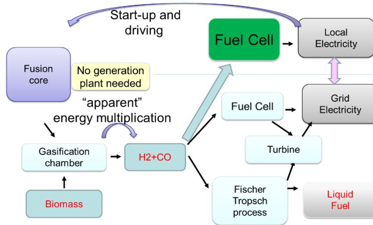
FIG. 1. Simplified flow diagram of energy use for Biomass-Fusion Hybrid. Electricity is mainly generated by the fuel cells at both local and centralized grids. Exhaust heat from Fischer Triosch process is used for turbine generator.
