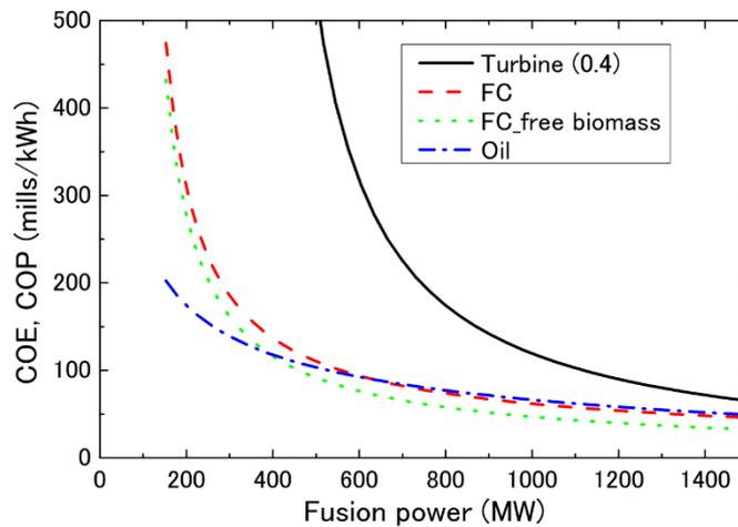
FIG. 2. Cost of the electricity from conventional turbine and fuel cells as the function of fusion power of a single reactor. Production cost for artificial oil is also shown at the equivalent product energy. Because the unit capacity of the fuel cells are small and thus modular, smaller generation is favourable for fuel cells.
