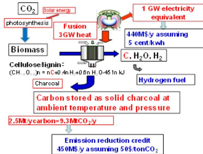
FIG. 4. Charcoal production by biomass-fusion hybrid plant.
