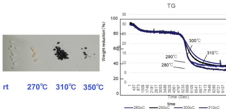
FIG. 3. Charcoal production from cellulose. Left: appearance of the reaction product against temperature. Reaction occurs at 310 degree completely, and above it sintering and weight loss of charcoal occurs. Right: Weight loss of cellulose heated at constant temperature increase. Reaction occurs at above 280 degree C.
