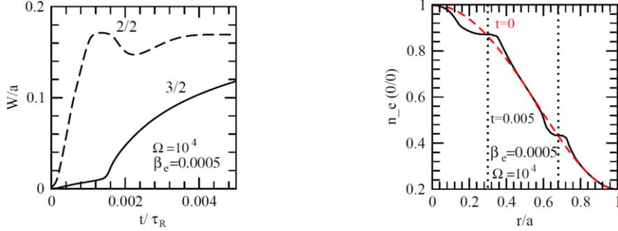
FIG. 1. (Left) Time evolution of the normalized  $2/2$  (dashed curves) and  $3/2$  (solid) island widths for  $\beta_e=0.0005/\Omega=10^4$ . (Right) Corresponding radial profiles of the normalized  $m/n=0/0$  component electron density at  $t=0$  and  $0.005\tau_R$ . The vertical dotted lines show the locations of  $r_{q=1}$  and  $r_{3/2}$ .
