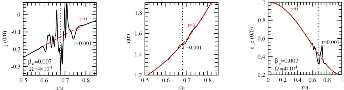
FIG. 3. For the parameters of the red curves in Fig. 2 (left), radial profiles of the  $m/n=0/0$  component plasma current density (Left), the safety factor (Middle), and the  $m/n=0/0$  component electron density  $n_{e,0/0}$  (Right) at  $t=0$  and  $0.001\tau_R$ . The vertical dotted line shows  $r_{3/2}$  location.
