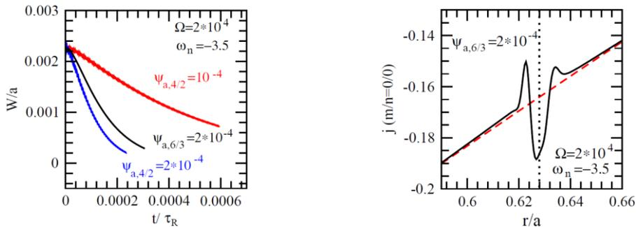
FIG. 8. (Left) Time evolution of the normalized 2/1 island widths with  $\Omega=2 \times 10^4$  and  $\omega_n=-3.5$  by applying static  $m/n=4/2$  or  $6/3$  RMPs. (Right) Corresponding radial profiles of the normalized  $m/n=0/0$  component of the plasma current density at  $t=0$  (dashed curve) and  $2.8 \times 10^{-4}$  (solid) for  $\psi_{a,6/3}=2 \times 10^{-4}$  and  $\omega_n=-3.5$ .
