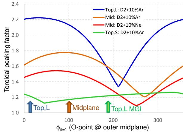
**Fig. 5:** Expected toroidal peaking factor for D<sub>2</sub>+10%Ar (orange) and for D<sub>2</sub>+10%Ne (red) from the midplane depending on the O-point position of a n=1 mode. The blue arrow indicates the toroidal location of the MGI.
