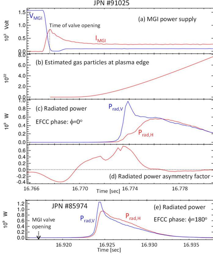
**Fig 3:** Time traces of the same discharge as in Fig 2: (a) response of the MGI power supply, (b) estimated amount of gas arriving at the plasma edge, (c) radiated power measured by the vertical (blue) and horizontal (red) bolometer and (d) the asymmetry factor of the radiated power. Box (e) shows the two measured radiated power for a pulse where the direction of the magnetic perturbation field has been inverted.
