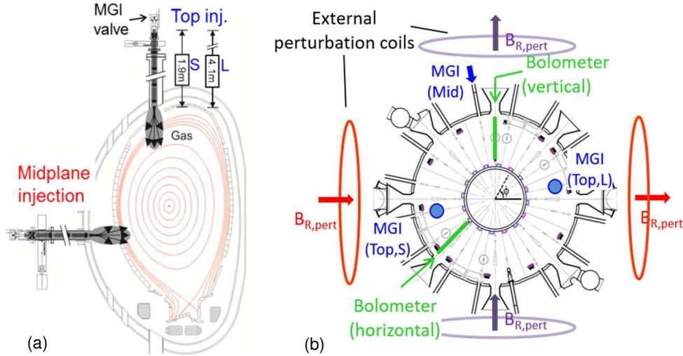
**Fig 1:** (a) Poloidal and (b) toroidal cross-section of the JET-tokamak showing the locations of the three massive gas injection valves and the horizontal ( $P_{rad,H}$ ) and vertical ( $P_{rad,V}$ ) bolometers. The red and purple circles indicate the toroidal location of the error field correction coils (EFCC). Note: the coils are not drawn to scale.
