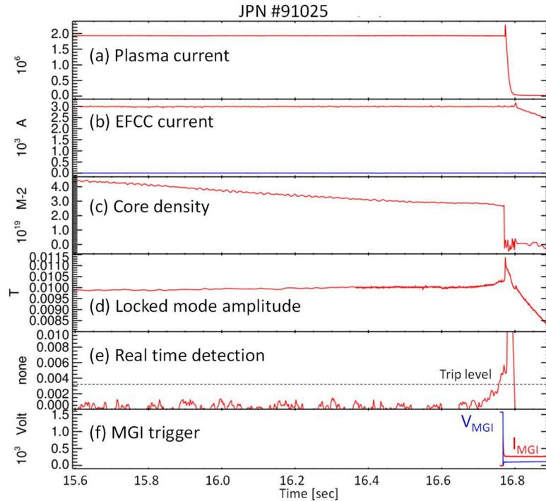
**Fig 2:** JET discharge with seeded error field mode: time traces of (a) plasma current, (b) EFCC currents corresponding to phase  $0^\circ$ , (c) line integrated plasma core density, (d) Amplitude of mode lock not corrected for magnetic perturbation field pickup, (e) real time detection of mode lock, (f) MGI power supply voltage and current.
