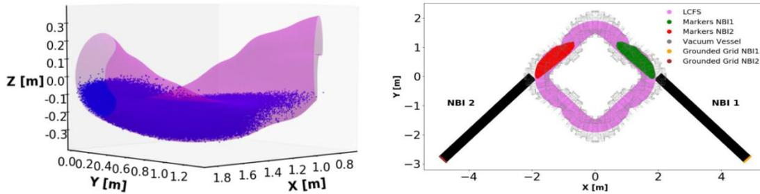
FIG. 3: Left: a 3D illustration of the ionization position of the co-injected initial markers representing beam particles and the last closed flux surface. Right: top view of the simulated neutral beams of TJ-II.
