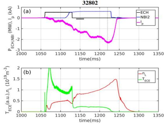
FIG. 2: (a) Time evolution of ECR and NBI heating powers and total plasma current of shot #32802. (b) Time traces of electron line-density and central ECE temperature. The plasma current does not evolve exponentially but linearly due to unstable plasma-density.
