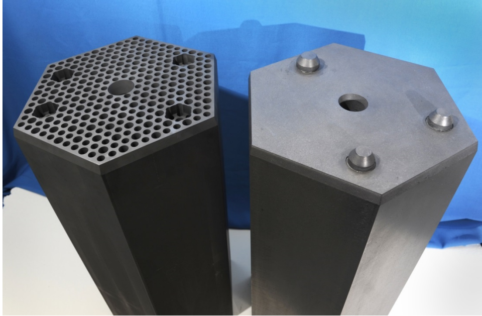
Figure 15. Typical prismatic fuel block (left) and a reflector block generic to both a prismatic and pebble bed design (right).
