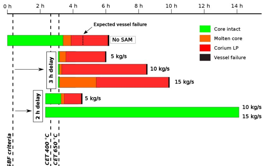
FIG. 4: Impact of secondary bleed and feed on the progression of the Station Blackout sequence. Vertical lines mark the occurrence times of major events for the SBO sequence without any SAM measure. Flow rates are referred to the injection rates into the depressurized SG i.e. SGB.
