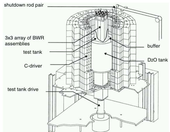
Fig. 2: The PROTEUS reactor at PSI with an insert of 9 BWR fuel elements, source: <http://proteus.web.psi.ch/facility/>
