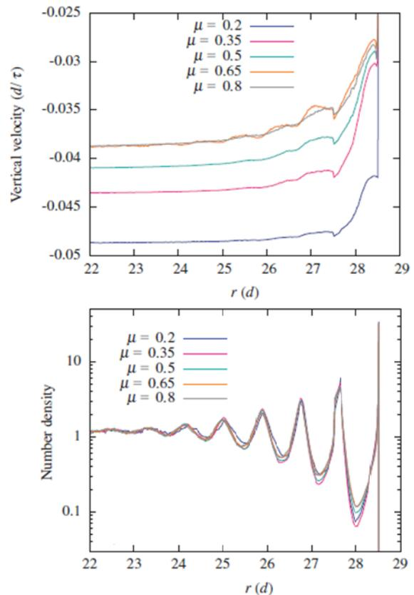
Fig. 12: Velocity profiles close to the wall (above) and growing order of pebble number density towards the wall (below), both as function of the friction coefficient  $\mu$ , [25]
