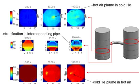
Fig. 8: MiniPanda generic air ingress experiment, temperature distributions measured by thermoresistive mesh sensors [22]
