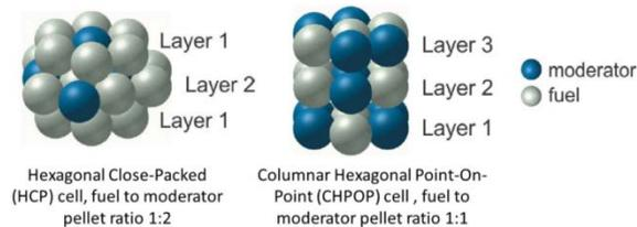
Fig. 4: Elementary cells of the regular pebble beds in the PROTEUS experiments [15]
