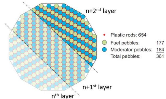
Fig. 5: Three successive layers of the core configuration of the PROTEUS core with polyethylene rods inserted in order to model moisture ingress
