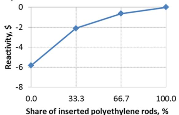
Fig. 6: Typical reactivity insert due to water ingress simulated by polyethylene rods
