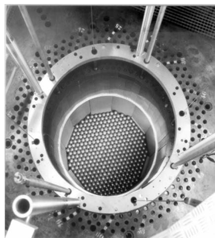
Fig. 3: The PROTEUS reactor with a regular loading pattern of pebbles, source: <http://proteus.web.psi.ch/facility/>
