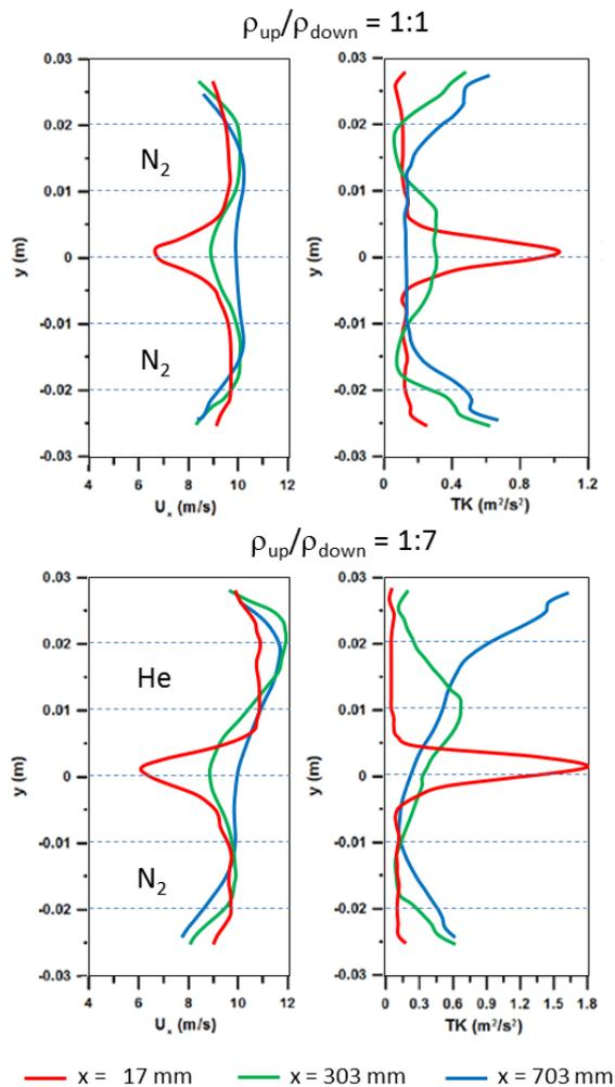
Fig. 10: Profiles of velocity (U) and turbulent kinetic energy (TK) obtained by PIV at the HOMER facility at equal velocities (8 m/s) and nitrogen in both inlets (above) and for a pure helium flow in the upper inlet and nitrogen in the lower inlet (below, density ratio 1:7),  $x$  = distance downstream of the rear edge of the splitter plate (from [23])
