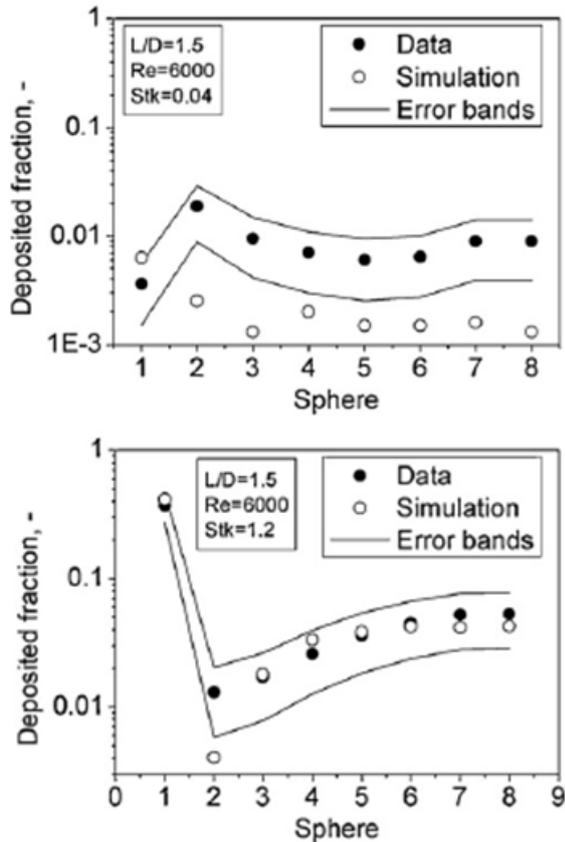
Fig. 15: Deposition of particles on a linear assembly of spheres at different Stokes numbers (from [27])
