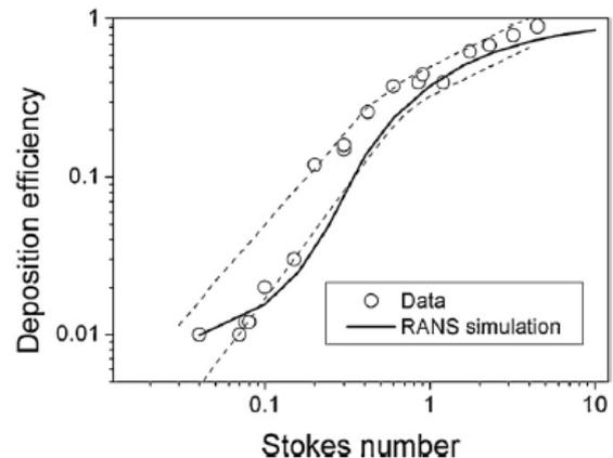
Fig. 14: Deposition of particles on a single sphere (taken from [27])
