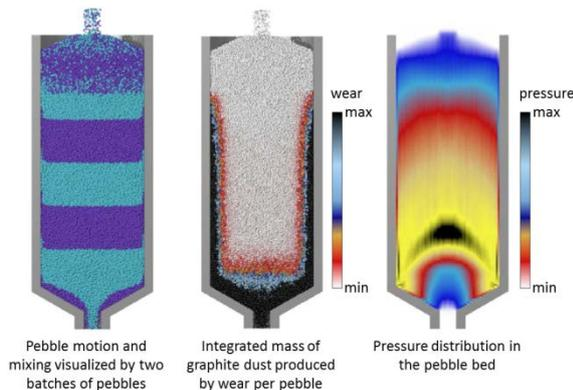
Fig. 11: Results of pebble flow and wear simulations in a generic HTR geometry (from [25])
