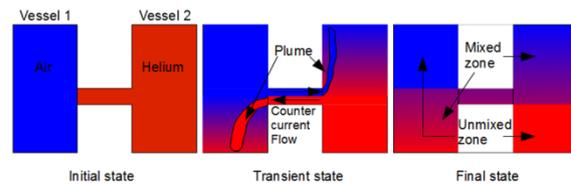
Fig. 7: Qualitative description of the generic air ingress experiment carried out at MiniPanda [22]
