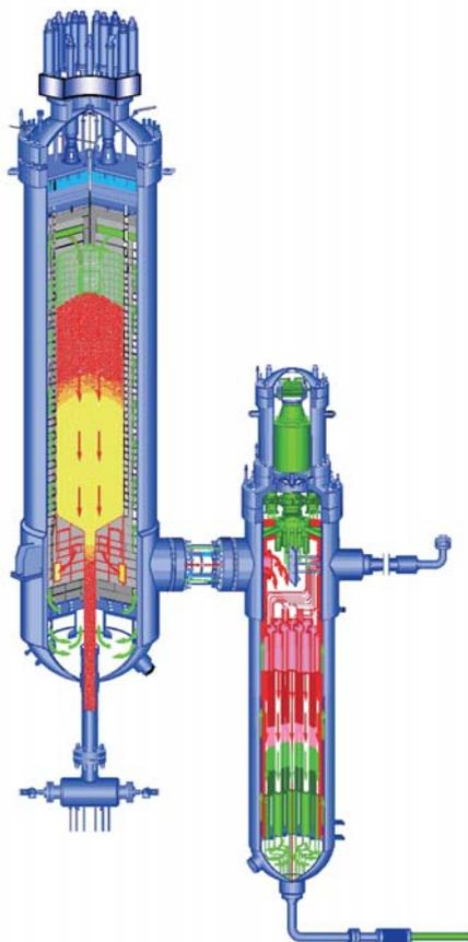
Fig. 1 Arrangement of reactor module and steam generator
