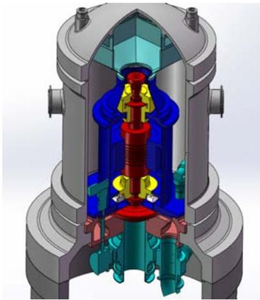
Fig. 4 Main helium blower on top of steam generator
