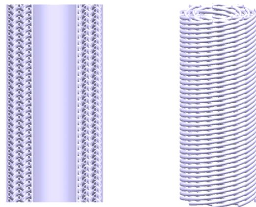
Fig. 3 Helical tubes in one assembly of steam generator
