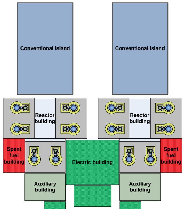
Fig. 6 Layout of 2 × HTR-PM600 nuclear and conventional islands
