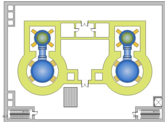
Fig. 5 HTR-PM reactor building as a basic unit for HTR-PM600
