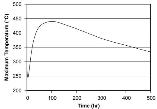
Fig. 9: Maximum reactor vessel temperature during nominal DLOFC event.
