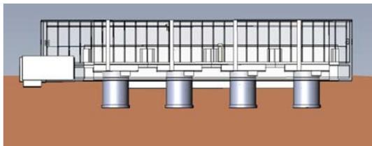
Fig. 13: Alternate four module SC-HTGR with partially embedded reactor buildings.
