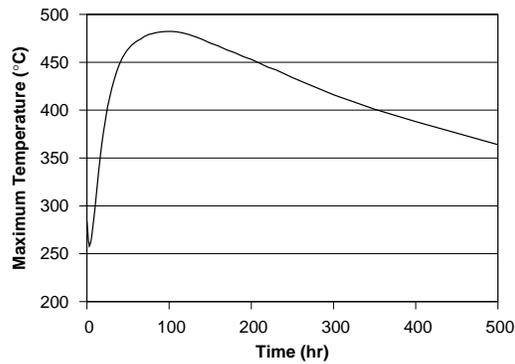
Fig. 11: RPV temperature DLOFC results for conservative RPV case.
