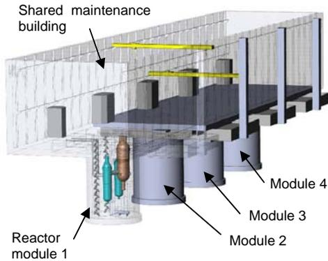
Fig. 6: Typical arrangement for four module plant.
