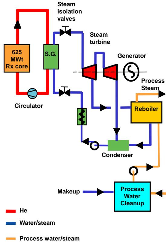
Fig. 4: SC-HTGR cogeneration system.
