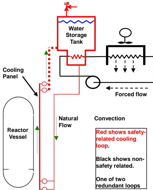
Fig. 5: Schematic of SC-HTGR Reactor Cavity Cooling System.
