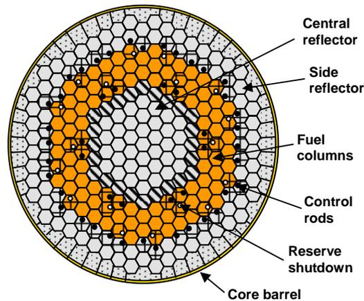
Fig. 2: SC-HTGR annular core arrangement.
