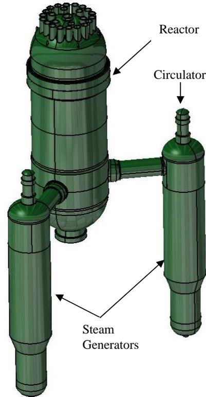
Fig. 1: SC-HTGR steam supply system.
