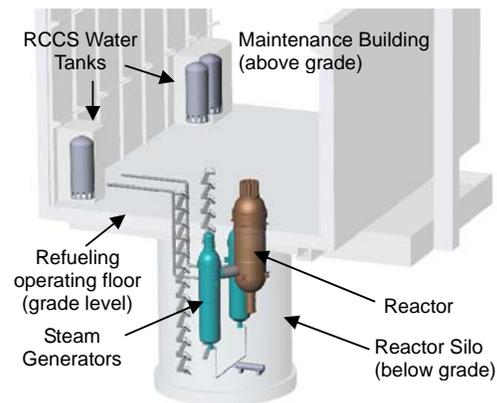
Fig. 3: Single SC-HTGR reactor module.
