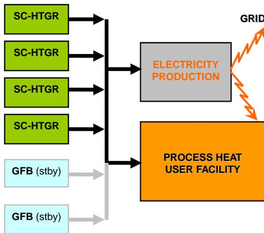
Fig. 7: Typical plant with SC-HTGR steam supply and natural gas-fired boilers (GFB) for backup.
