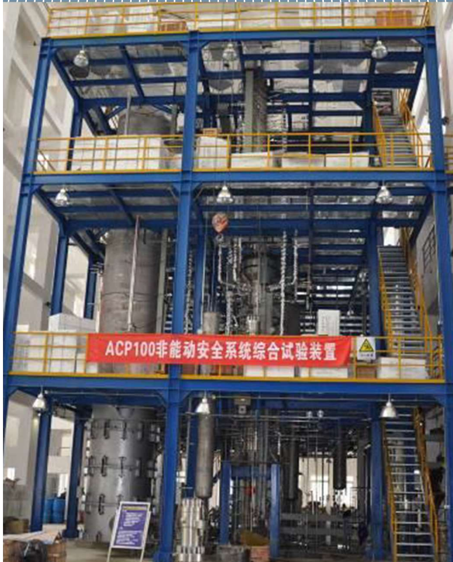
Core Cooling and REsidual heat removal System Test facility (CREST)
