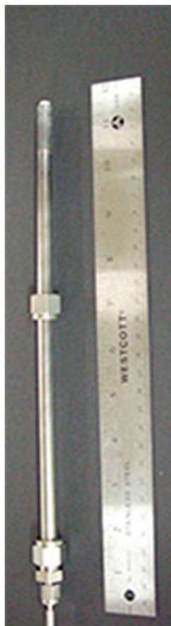
FIBER OPTIC sensor (T)
