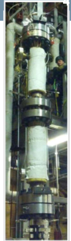
NuScale: CHF test section (Stern Labs)
