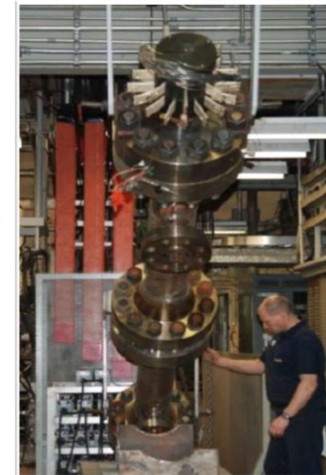
SMART: CHF test section-freon (FTHEL facility)
