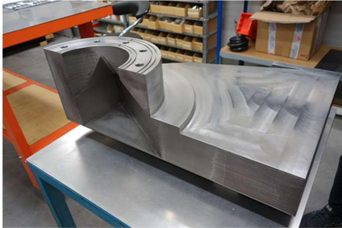
Compact SG: set of mock-up to set-up the manufacturing process
