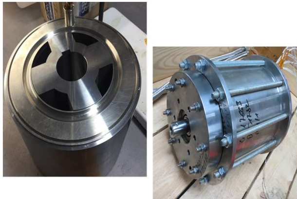
Electrical CRDM : Two hermetic technologies of motor under high temperature testing
