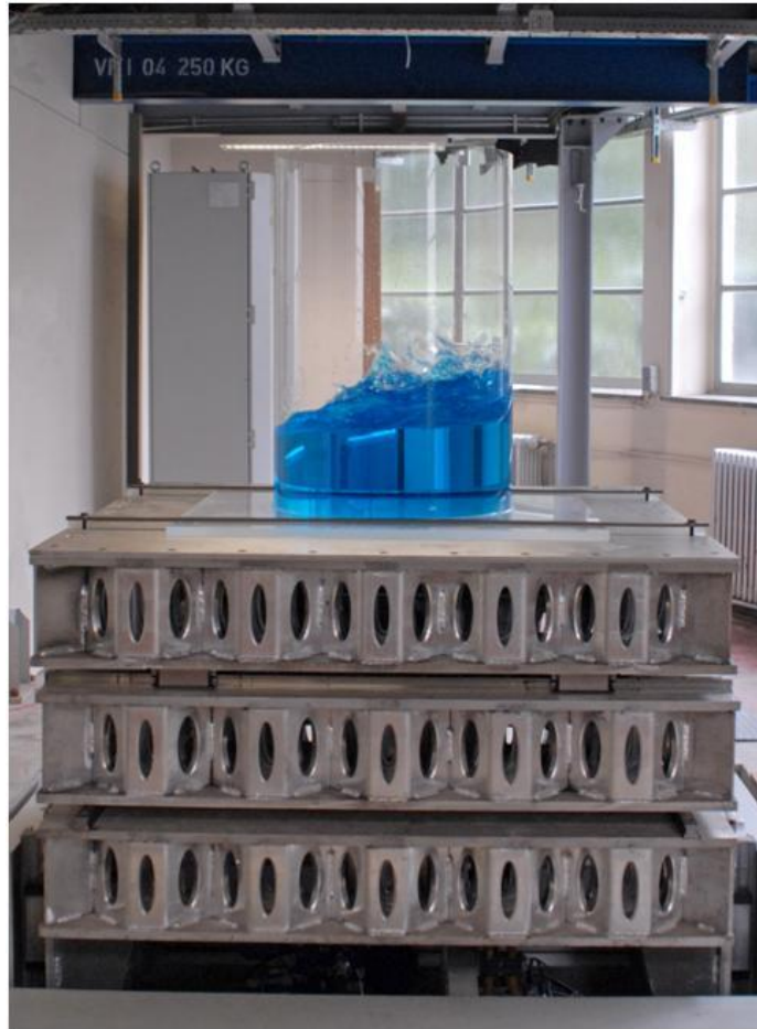
FIG. 2. Experiment of sloshing in cylindrical tank on the SHAKESPEARE facility.
