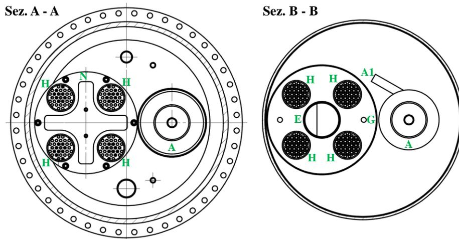
FIG. 3. CIRCE vessel and SGTR-TS horizontal sections A-A and B-B
