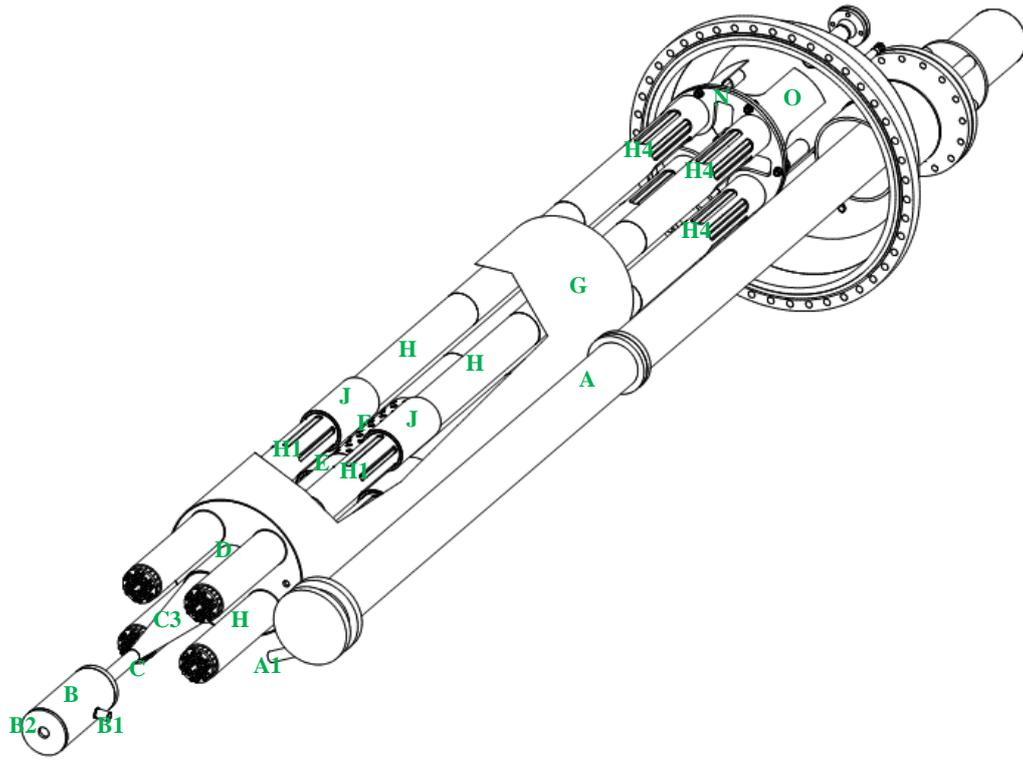
FIG. 1. SGTR test section, 3D bottom view
