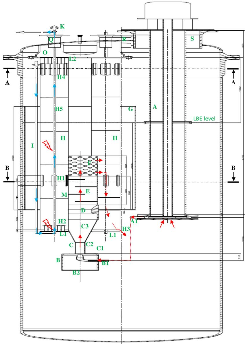
FIG. 2. CIRCE and SGTR test section, 2D vertical section (out of scale: height conserved, width enlarged 5 times)
