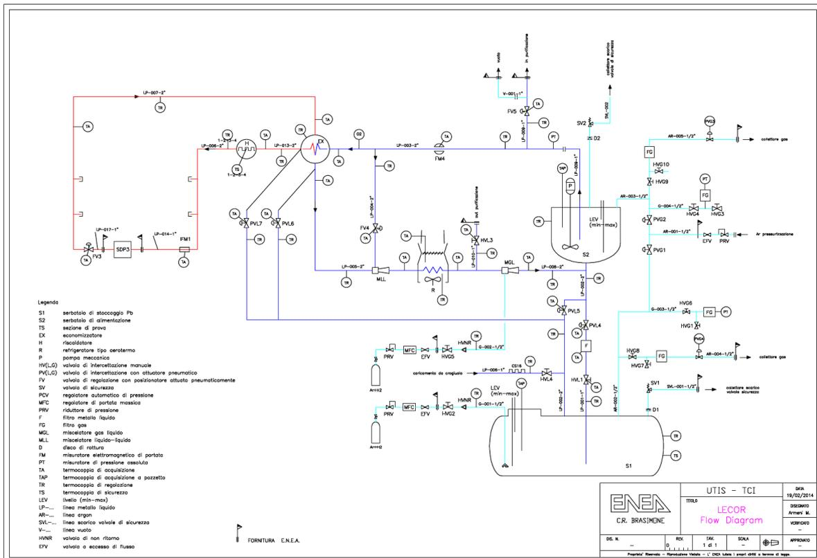
FIG. 1. Scheme of the LECOR facility
