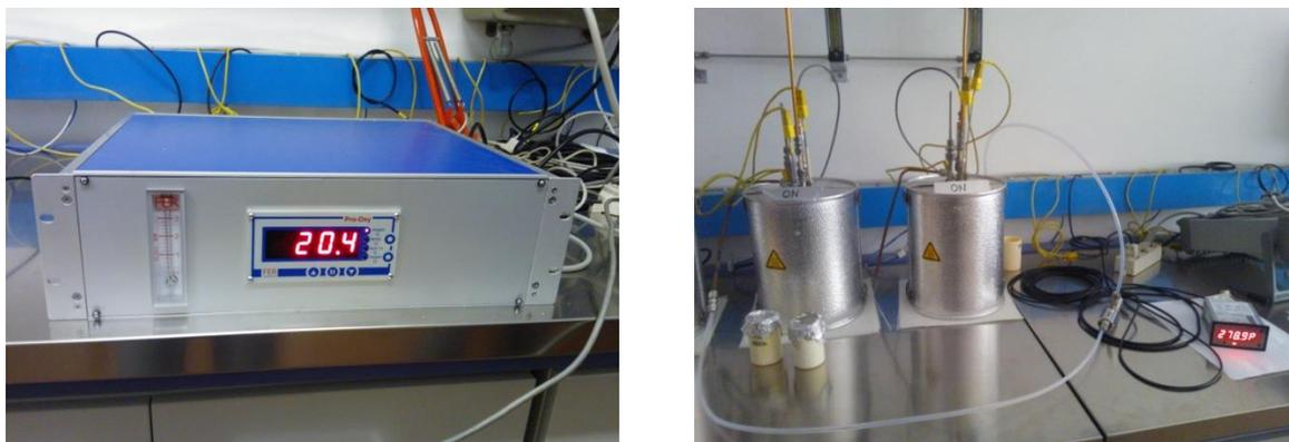
FIG. 2. Instruments for chemical control in gas, a) oxygen gas analyzer during calibration in air and b) hygrometer for the monitoring of water production in the cover gas out coming from KIT devices.
