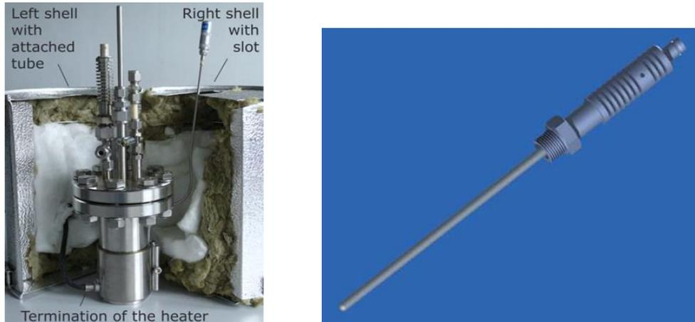
FIG. 1. Images from Ref. [1] showing a) KIT experimental capsule without insulation components and b) KIT oxygen sensor for corrosion tests in liquid lead at high and low oxygen content.
