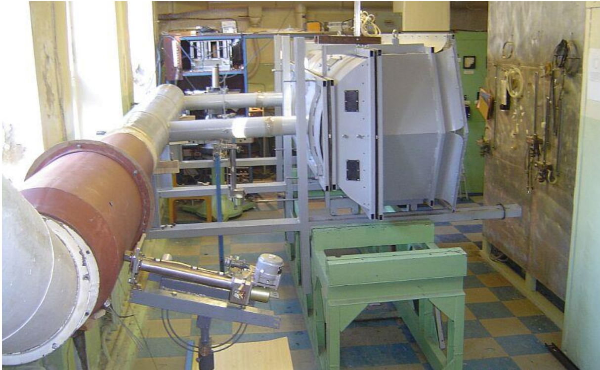
FIG. 2. Perforated steam-distribution plate (VVER-1500) test model in the circuit of the aerodynamic facility "B-2"
