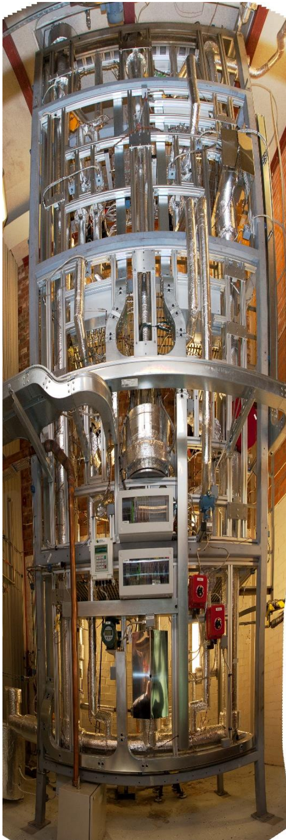
FIG. 2. TALL-3D primary side, pin-like Main heater and pool type Test section
