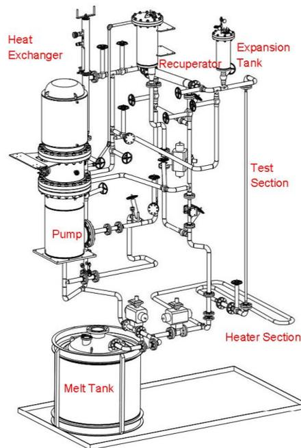
FIG. 1. Scheme of the DELTA facility
