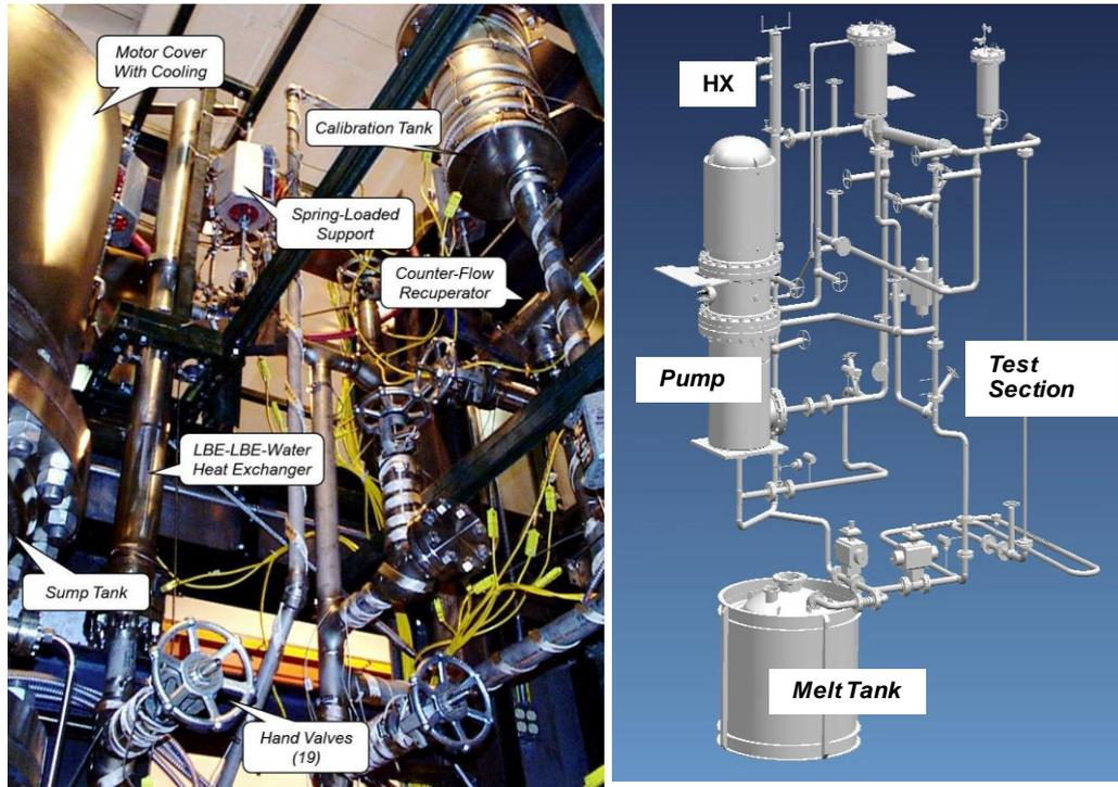
FIG. 2. View of the DELTA facility (left) and its 3D drawing (right)
