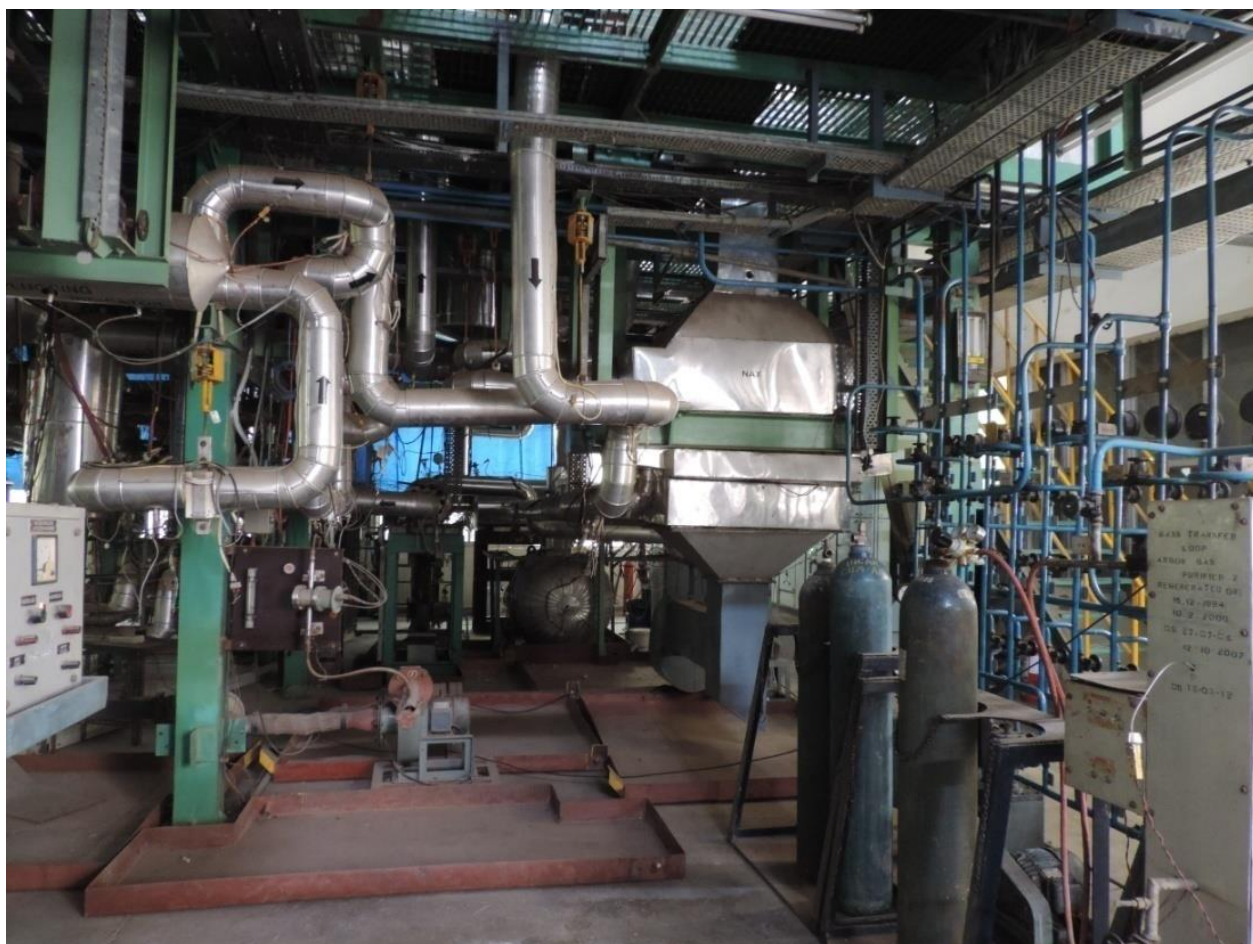
FIG. 2. BIM Loop Pipe Lines and Components
