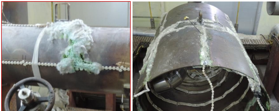
FIG. 4. Test sections after sodium leak experiments
