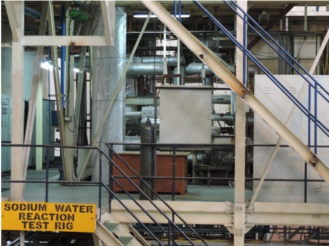
FIG. 3. SOWART Structure with loop pipelines
