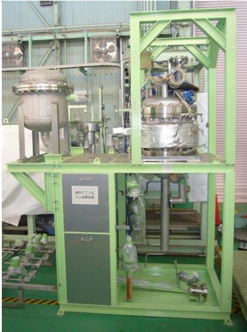
FIG. 2. View the MELT test section for sodium experiments to study fuel-coolant interactions
