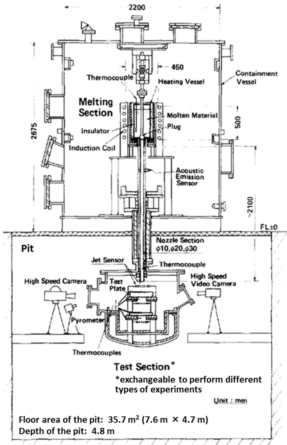
FIG. 1. Scheme of the MELT facility
