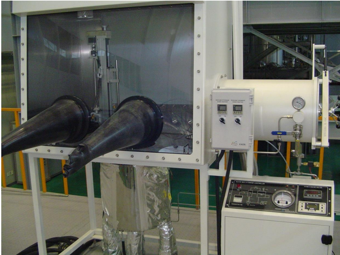
FIG. 3. Glove box and argon circulation/cooling system
