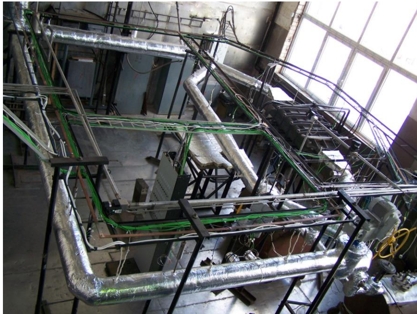
FIG. 3. View of the sodium loop DN 125 "TESLA"
