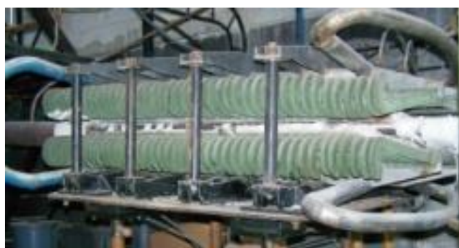
FIG. 2. View of the flat induction pump under investigation at TESLA ( Q up to 70L/s; p =5bar)
