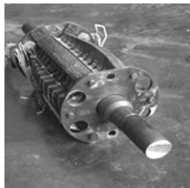
FIG. 4. Annual EMP with Nb made channel, tested temperature up to 1150K
