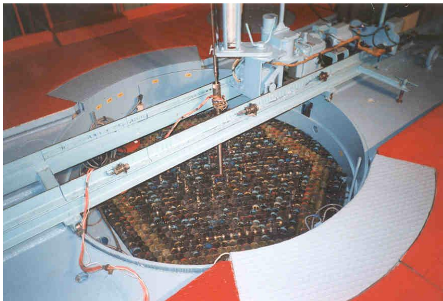
FIG. 3. Upper part of the «BFS-1» facility with the measuring device
