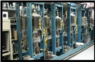
Creep frames with Inert environment
